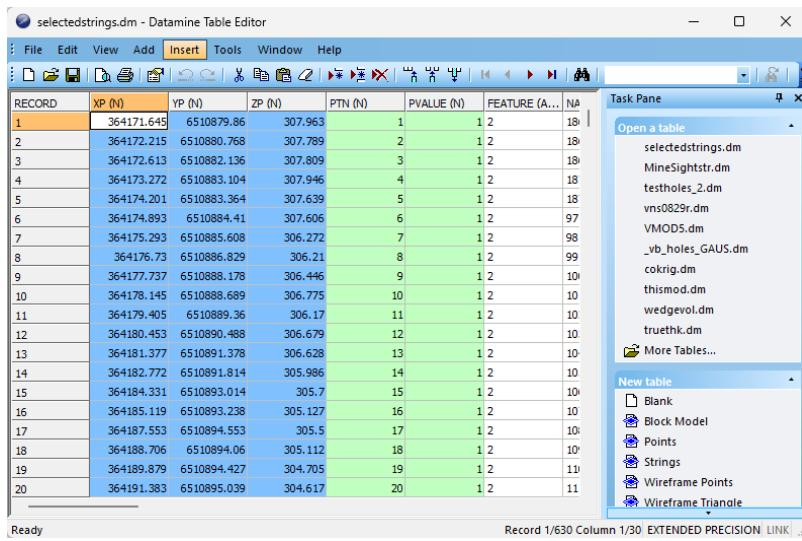
The Datamine file format used natively by Studio products originated from Datamine's "Native File System" over thirty years ago. It has been maintained and supported by Datamine products since then. The mining industry has seen a significant increase in data volume and complexity during this time, which has started to strain the capabilities of the Datamine format.
