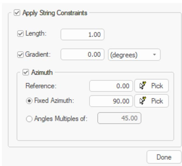
This can help to ensure operational and design constraints are honoured during digitizing, saving time later by editing and adjusting design data. Help files for both commands have been updated to explain how to use the new controls. You can also press F1 when the new popup displays during digitizing.
